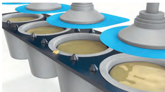
watttron detects product residues, double or missing lids directly during the sealing process, ensuring maximum process reliability.
