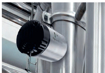
In-Line NIR Analyzer in Operation.
