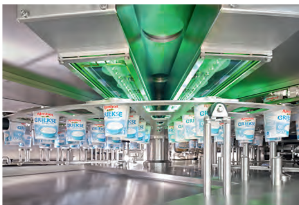
High-energy radiator of the two-stage pulsed light high-performance UV(C) sterilisation process in the hygiene tunnel of the 4-lane cup filling machine GRUNWALD-ROTARY 20.000UC. Photos: Grunwald
